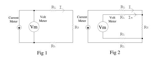
This is why a 2-wire tester is inaccurate for measuring low resistance's (fig 1). R<sub>s</sub>: -Resistance of sample (e.g. Cable or Harness) R<sub>L</sub>:-Resistance of lead V<sub>M</sub>: - Measured voltage
